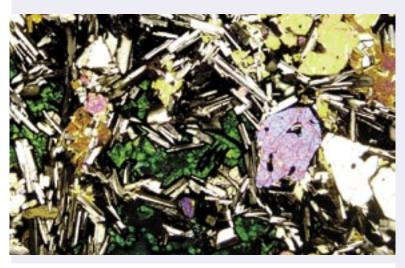
Figure 1 – Petrographic micrograph of basalt in thin section (stained with methylene blue) showing volcanic glass (dark areas) undergoing alteration to deleterious smectite clay (dark green). Crossed-polarised light, width of field: 3.5 mm.
