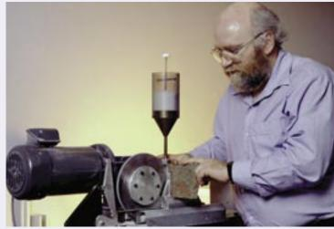
Figure 2 – Determining abrasion resistance of stone using: (a) the Taber abraser method; and, (b) the Capon method.
