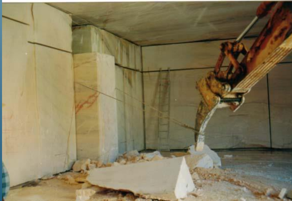
BLOCK PULL OUT BY MEANS OF BACK-HOE EXCAVATOR
